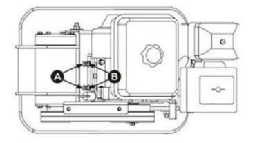
8.30 Push the engine toward the back of the plate by turning the adjustment bolts A to remove any slack in the V-belt(s).
