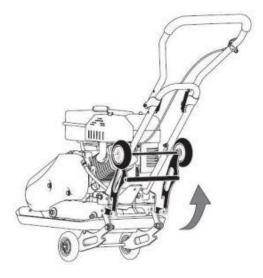
3.6 Attach the paving pad (if required) by aligning the holes on the base plate with the holes in the paving pad and mounting plate.
