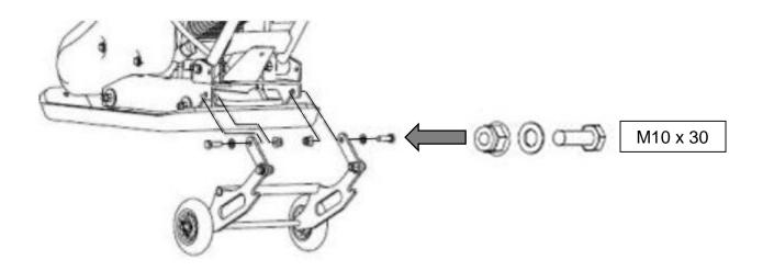
3.5 Before using the compactor plate, you **MUST** fold up the wheel kit.
